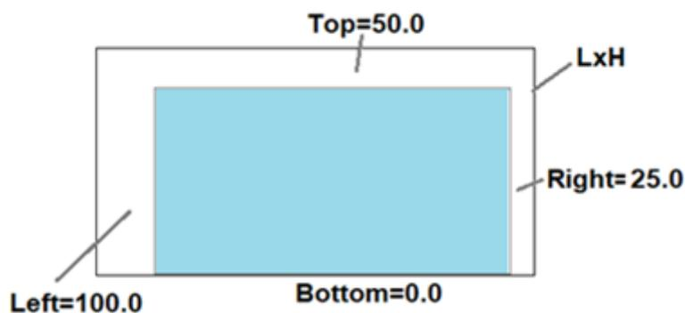
The outer margins setting corresponds to [OneSheet](#) structure fields: BorderLeft, BorderRight, BorderTop and BorderBottom.
