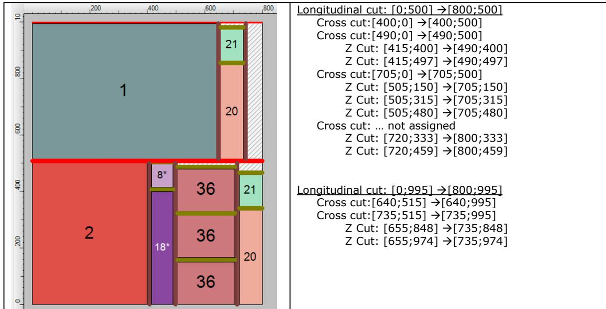
The last *cross cut* reported for the first *longitudinal cut* is indicated as "not assigned" as it is completely outside the right edge of the sheet.
